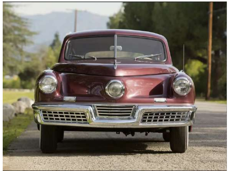
Caption for front end Lights: Sealed Beam Headlamps with Center Rotating "Cyclops Eye"
