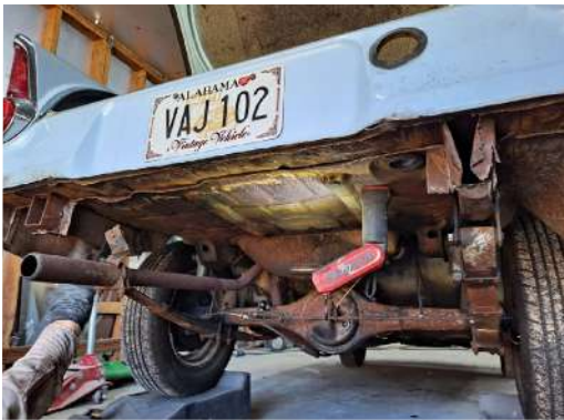
Figure 1: Gas tank out, valence removed.
