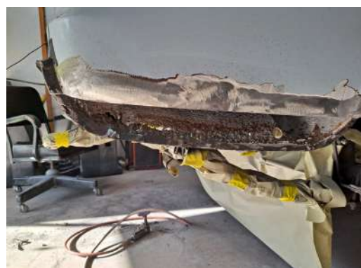
Figure 6: Rear passenger quarter panel ready for new metal
