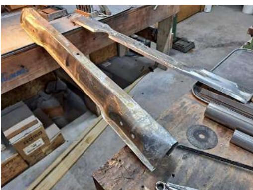
Figure 5: Rear cross member and valence prepped for installation
