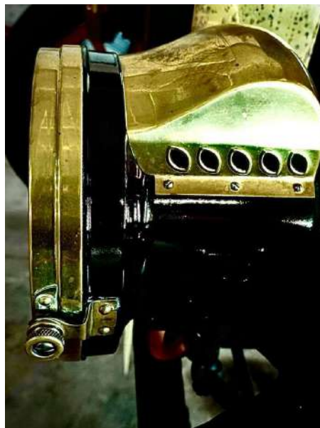
Carbide lamp of the 1914 Pie Truck!
