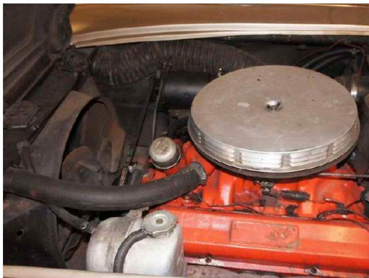
The original 327 cubic inch engine producing 300 horsepower powers Ann-Shirley Goodell's 1962 Corvette.
