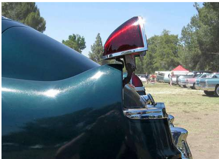
The left taillight is hinged, flipping up to reveal the fuel filler. Cadillac first adopted this feature in 1941. Not only was it a conversation piece, it obviated the need to clutter up the fenders with a conventional fuel filler cap.
