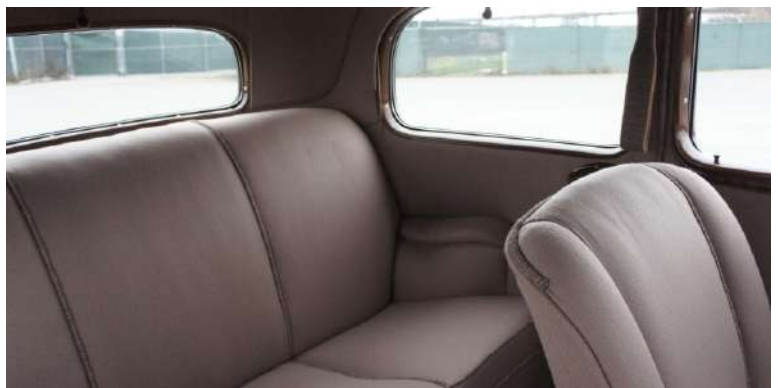
Original style material was used to reupholster the 1933 McLaughlin Buick Victoria with detail down to the tassel and string attached to the side window blinds.
