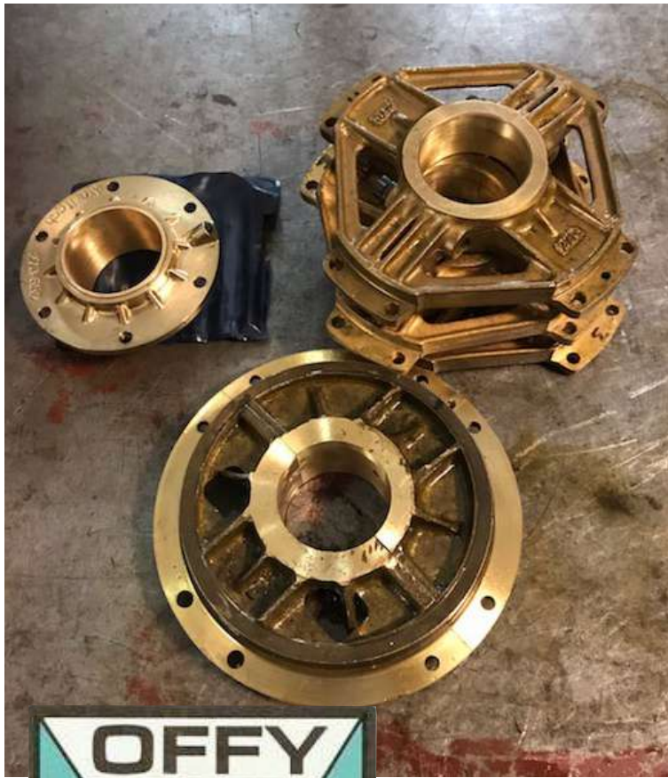
Above: Brass crankshaft front and rear bearing supports and the girders are also bearing supports for the engine
