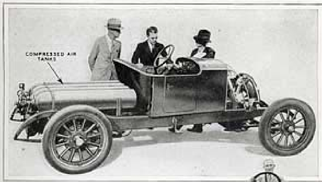
A side view of the compressed air car, showing the four fuel tanks which will drive the car 500 miles at a speed of 35 miles an hour. The engine requires no cooling system, no ignition system, no carburetor, nor the hundreds of moving parts included in a standard gasoline motor.
