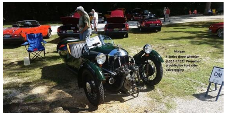
Morgan F-Series three-wheeler (1932-1952). Propulsion provide by Ford side valve engine
