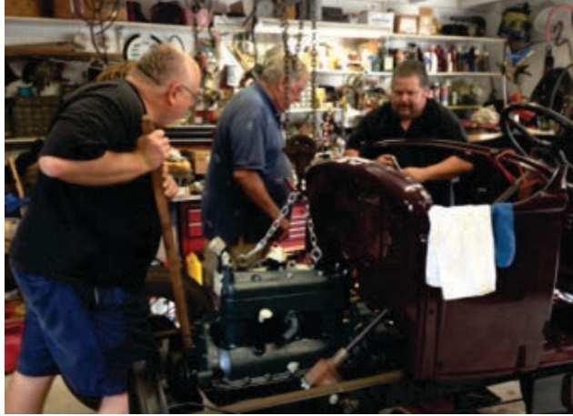
Zeno and Rick help Walt put the motor in the Model A.
