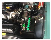
I reinstalled the generator and took it back for them to check out the car. After the two older gents argued for a while about the nature of the voltage output, it was decided that the idling charge was a little over 12 volts and that it got up to around 14.1 volts when they put up the rpms. It was suggested that I get a smaller pulley on the generator so it would spin faster to get the idle voltage up. The evil alternate was to replace it with an alternator.
